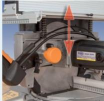
New upper table adjustment by cranted system. Gives a precise and smooth adjustment.
