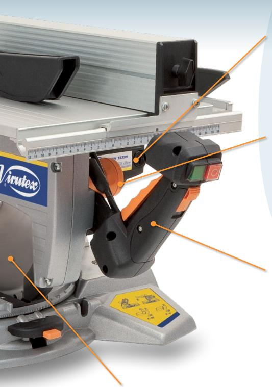
Easy change of saw blade thanks to the blocking button. Equipped from factory with a carbide saw blade d. 300 mm 48 Z. Electronic circuit protecting the machine against unintentional switch on due to a power supply lack. It also allows the soft start of the machine, without sudden jerks avoiding breakdowns on belts or moto.
