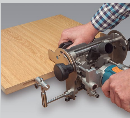
Trimming at 90° using the guide
