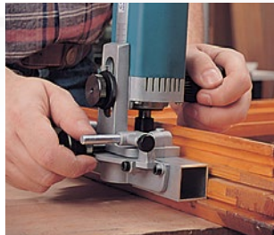
Slotting a window, flashing side.
