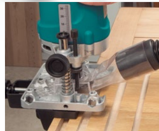
Slotting wood or plastic materials.
