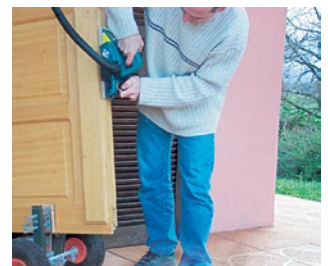
Wheels can be blocked for a stationnary use, so it is possible to work on the edge of the panel or the door.
