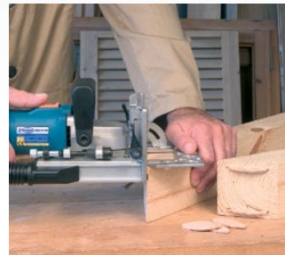
Stronger joints with No. 6 splines.
