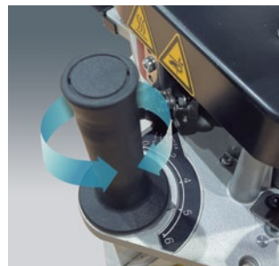
Speed adjustment controlled by microprocessor.
