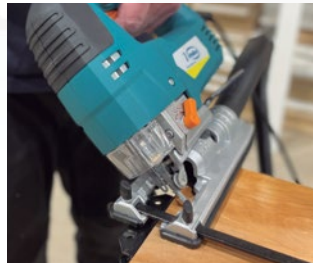
Base can be tilted from 0° to 45°.
