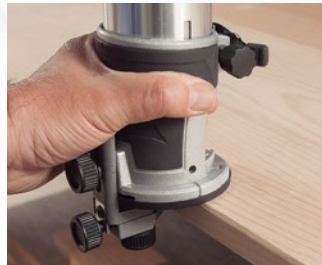
Realization of chamfers or moldings.
