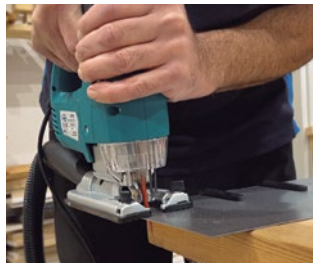
Metal sheet cutting.
