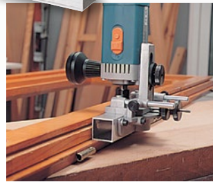
Slotting a window, hinges side.
