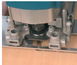
Guide ring for copying with template as a small router.
