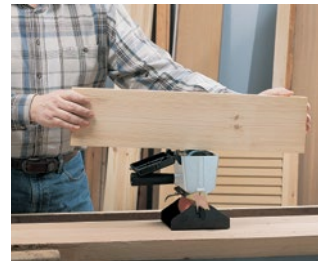
Gluing with the upper roller.
