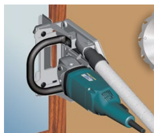
Trimming wooden window frames. Register on the adjustable front guide square.
