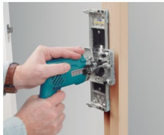
With help of the square guide with milimetric adjustment it's possible to cut perfect mortises for door hinges.
