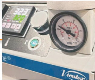
Self-regulated compressed air pressure.
