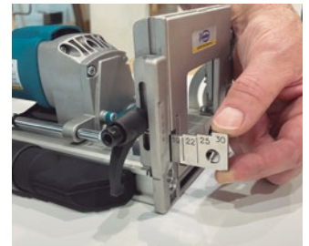
The panel thickness adjustment is very easy and intuitive.
