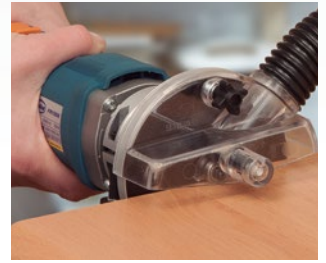
Round head for profiling with support on the edge.
