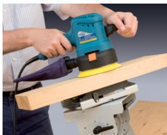
Folding and rotary adjustable support.
