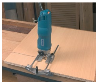
Trimming parallel slots.
