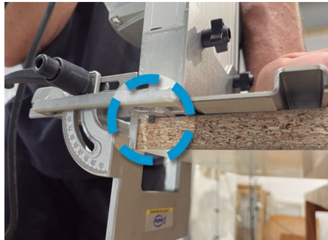
Automatic positioning system of retractable stoppers.
