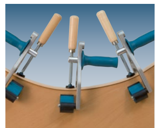
Fixing tapes on concave panels
