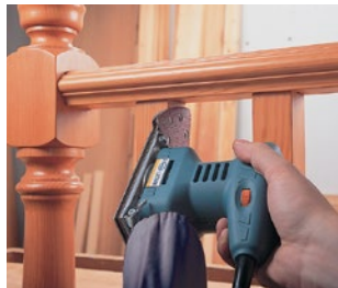
Using the delta base interior corners are quick and easy to sand.
