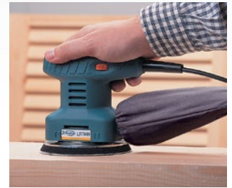
Like rotary orbital it combines two movements: rotary and orbital.
