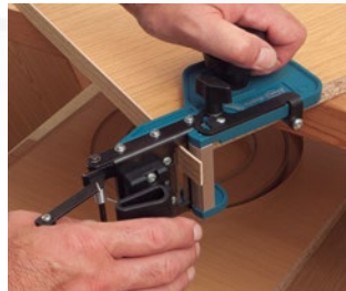
Cutting on both sides on straight panels.
