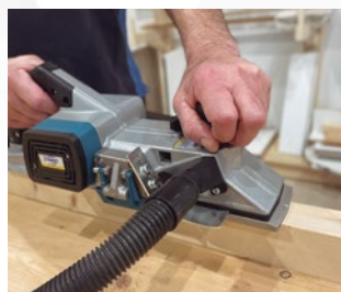
Dust collector connection.
