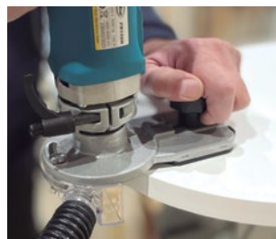
The CA56U trimming head enables uninterrupted trimming of the four edges of a panel. It has a large support base and an auxiliary holding knob, designed to give it perfect stability.
