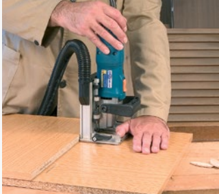
Joints in middle of board.
