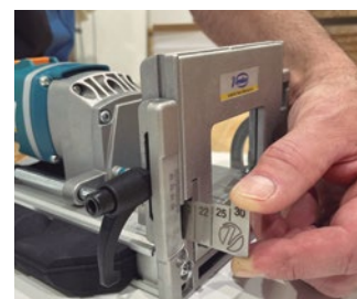
The panel thickness adjustment is very easy and intuitive.
