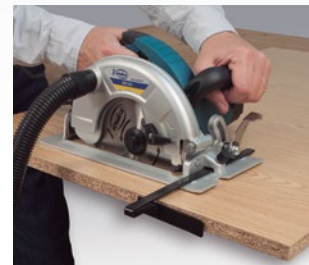
Light and stable, can make cuts of up to 55 mm.
