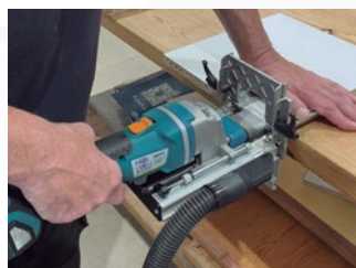
Easy and fast drilling on the edge of the panel, at 90° and 45°.
