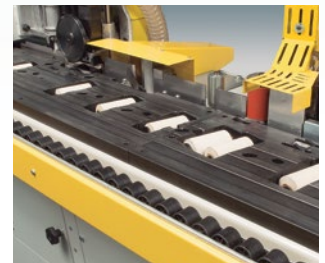
Equipped with auxiliary rollers on the banding table and a presser assembly, to achieve the optimum pressure of the panel against the banding unit. This ensures a correct banding.
