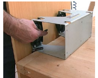
It is possible to hold panels in horizontal or vertical position.
