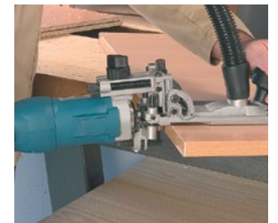
Trimming the edge with the straight bit.
