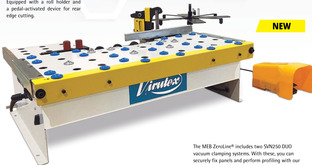
Edgebanding of straight, shaped, or beveled panels (up to 45°).
