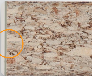
Glue line with others edgebanding technologies
