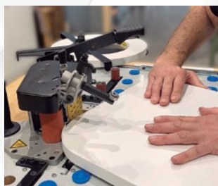
Edgebanding of straight, shaped, or beveled panels (up to 45°).
