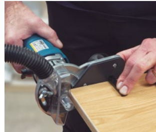
Precise guidance for corner profiling.
