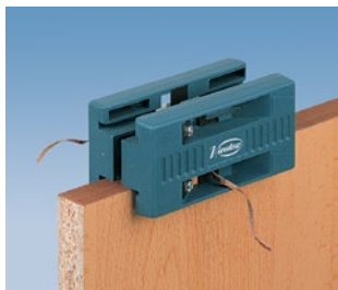
Trims both sides simultaneously.
