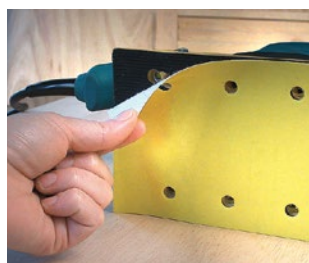
Mobile base for use with velcro sandpapers.
