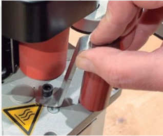
Auxiliary roller for 90° edgebanding. Can be positioned in two different settings depending on the piece being edged.
