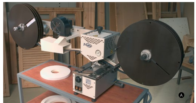
Easy access glue tank on top. The glue application system includes an easy, non-stick silicon roller.
