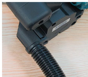
Dust collector connection.
