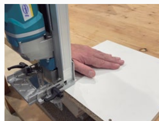
Easy and fast drilling on the edge of the panel, at 90° and 45°.
