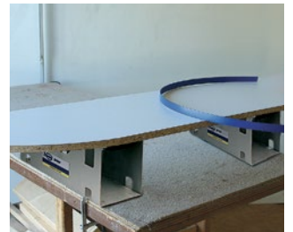
Using two vacuum tables it is possible to hold larger panels.
