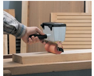
Gluing with vinyl (white) glues
